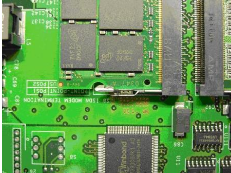
Figure 185: Fastening memory module in CP PM card
